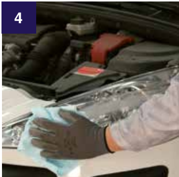
4 Check results every time sanding grid is changed, clean between sanding steps with SprayMax Wax & Grease Remover
